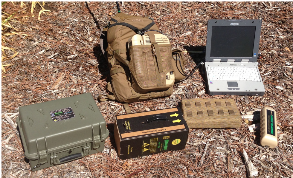
Figure 1 - XX55 fuel cell with micro-manager in backpack operating a 117G radio, charging a BB2590/U battery and operating a rugged laptop: also shown are various fuel cartridges compatible with the fuel cell
